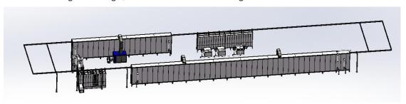
Complete System Includes: Spraying Treatment, Drying Oven, Autimatic Powder Spraying Equipment, Powder Coating Booth, Curing Oven, power and free conveyor
